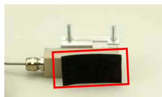
Picture 6 Using acoustic coupling foil
