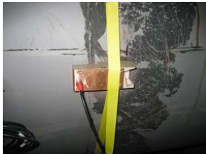
Figure 18: Textile tension bands are recommended for the assembly of the DUC-WP05 transducers (temperature limitation)
