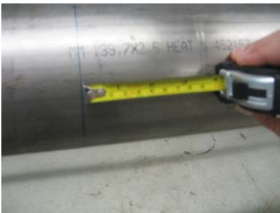
Figure 9: Mark the distance between transducer
