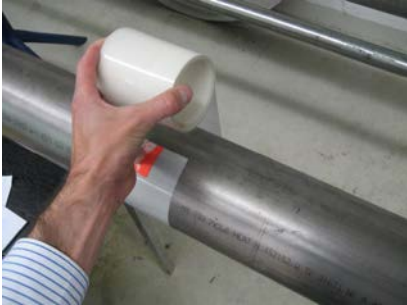
Figure 7: Attaching the template tape
