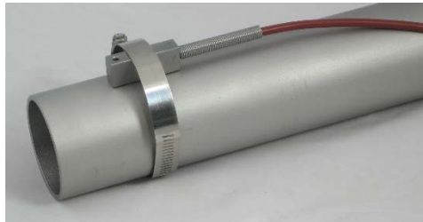
Figure 22: At pipe mounted Pt100
