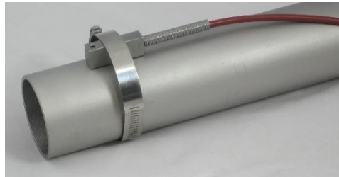
Figure 22: At pipe mounted Pt100
