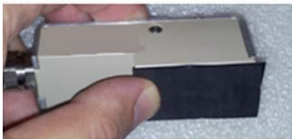
Figure 10: DUC-WF10 with acoustic coupling pad
