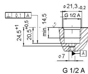
Screw in hole/Screw in socket for flush front diaphragm with o-ring sealing
