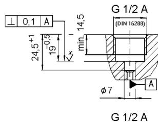
Sealing with flat gasket ring
