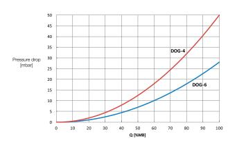
The diagram applies for gases with a density of air at NPT (0°C and 1013.25 mbar). The pressure loss is always proportional to the density of the gas. For example, the pressure loss doubles at 100% higher operating pressure.
