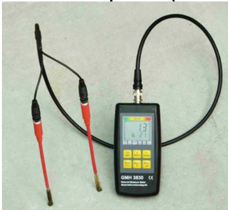
Measuring concrete with brush probe HND-FF06
