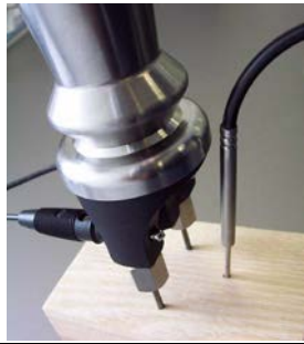
Reciprocating piston electrode HND-FF01 with temperature-probe –FF10
