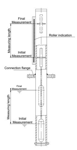
Remove the cotter pin from bottom end of the dip pipe, next, remove the transport lock of the float. Fix the float with the magnet system towards top and make sure, there are no remains of packing material or other impurities inside the tube.
