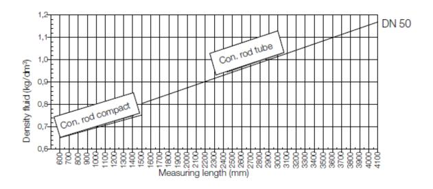
NBK-04 ...6: Float: titanium Connecting rod: titanium
