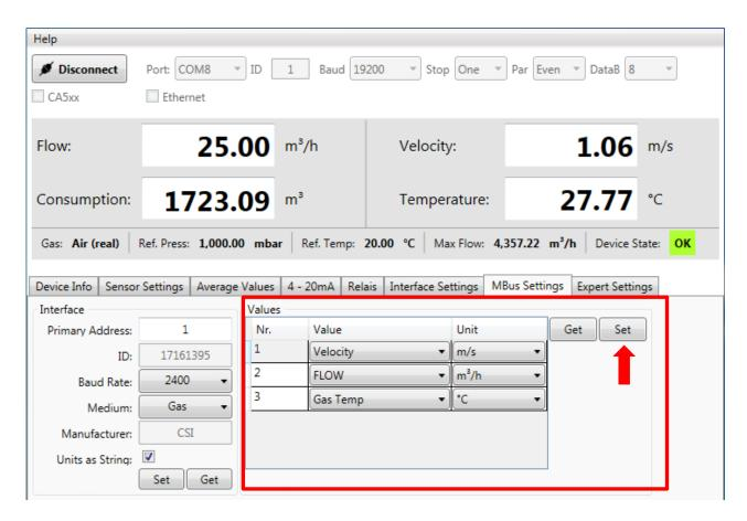
Basically, production setting is the "Fixed Data Structure" transmission mode, means 3 values with defined units will be transferred.
