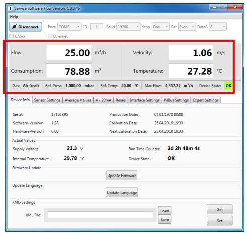
The upper part of the window shows the current measurements. In this case the calculation of "Flow" and "Velocity" are based on the values "Reference pressure" and "Reference temperature".
