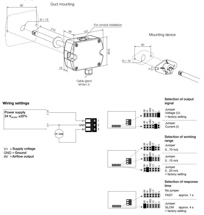
The output signal, working range and response time are selected via the jumpers according to the picture.
