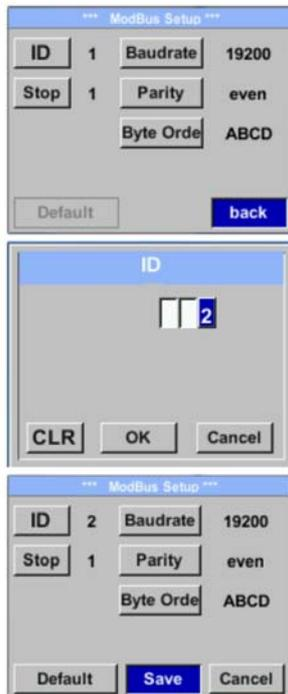
For changes, e.g. the sensor ID, first select by pressing key „△“ the field “ID” and then key “OK”.
