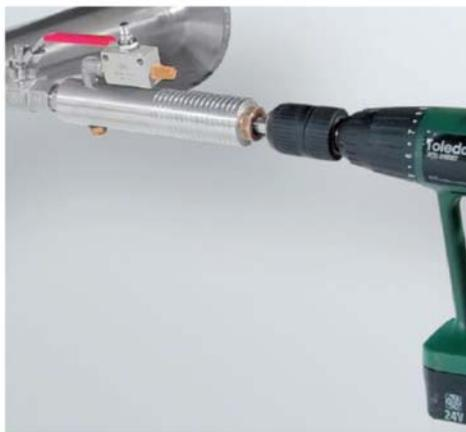
In case the system could not be shut down, means to be set depressurized, there could be used a spot drilling collar and drilling jig (on request) to drill through the ball valve.
