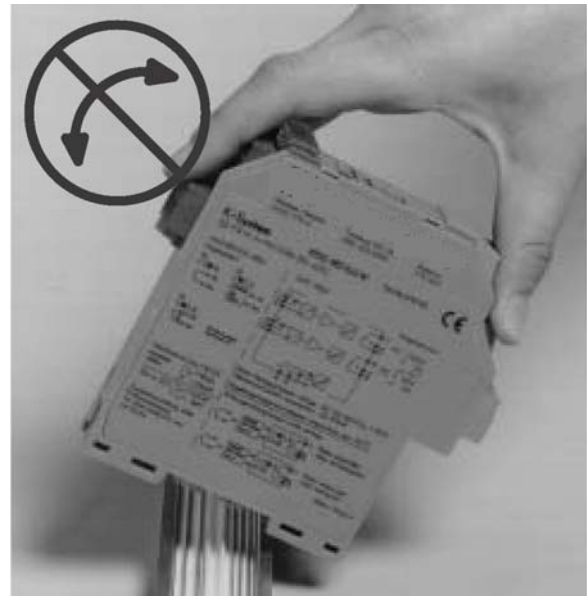
INCORRECT: Unit snapped on at an angle.
