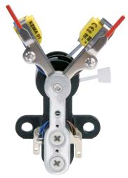
These contacting devices switch free of delay in the same way as the motion of the actual-value pointer. They should be used where no contact loading is required and the instruments are not exposed to vibrations. Due to sparking the contacting devices should not be used where there is a danger of explosion. Care should also be taken that the contacting devices are not exposed to the effects of aggressive vapours.
