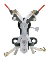
Pneumatic limit signal transmitters work without contact and with a very low feedback onto the mechanical pressure measuring system. They do not generate any electrical contact problems like wear, welding or excessive contact transfer resistance. Pneumatic contacts are used where controls work using pneumatic regulation and require high reliability and switching frequency, i.e. a longer life.
