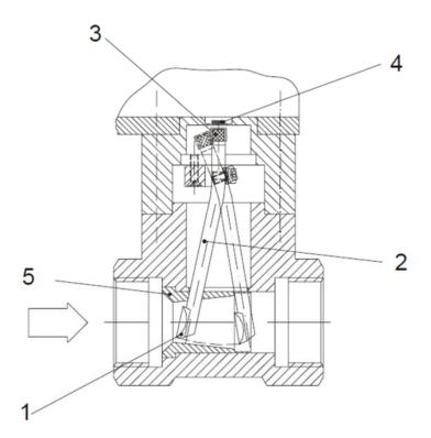
When the diaphragm plate is moved by the flow in the flow direction, the lever arm is deflected by the force of the leaf spring.
