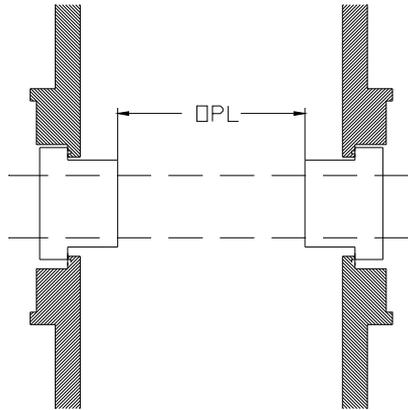
Due to the modular concept of the sensors, it is easy to change the optical pathlength (OPL) by changing the windows used:
