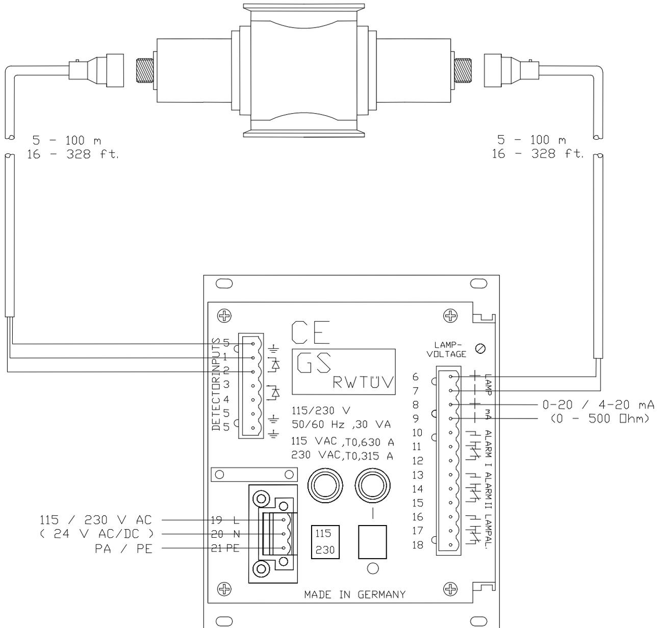
The system consists of two components, the converter type ATT-KA and the sensor type ATA-K which are interconnected with two cables (max. 100 m / 328 ft). Concerning the sensor, it is impossible to cross connect the cables, as different plugs are used. (9-pole on the detector side, 4-pole on the lamp side). The detector cable is not compatible with former version cables with an 8-pole connector!!!
