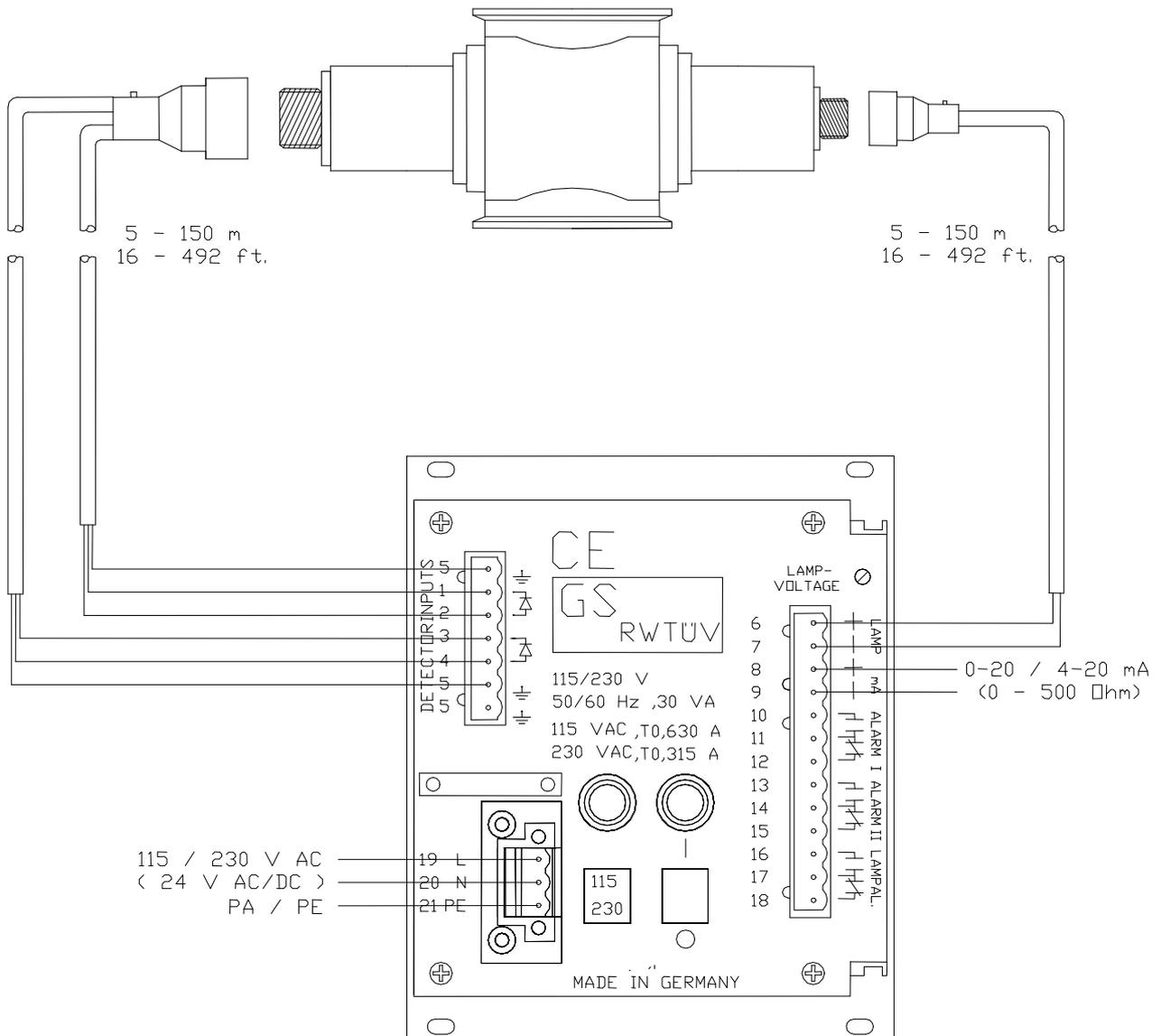
The system consists of two components, the converter ATT-KS and the sensor ATS-K which are interconnected with three cables (max. 150 m / 492 ft). Concerning the sensor, it is impossible to cross connect the cables, as different plugs are used. (9-pole on the detector side, 4-pole on the lamp side). The detector cable is not compatible with former version cables with an 8-pole connector!
