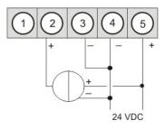
DAG-A4V ... in combination with a 3-wire-sensor 0 \_10 V
