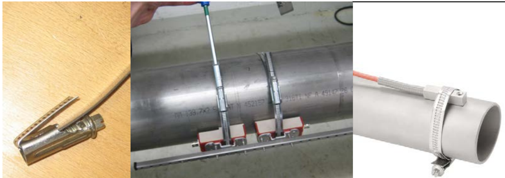
Pictures 7 Mounting DUC-WF Transducers, PT100 with stainless steel belts on a pipe
