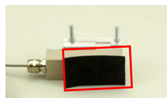
Picture 6 Using acoustic coupling foil
