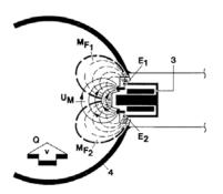
MF1, MF2: magnetic field E1, E2: electrodes 3: coils 4: pipeline U<sub>m</sub>: induced voltage
