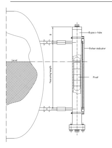
Remove the bottom flange from the bypass tube, and insert the cylindrical float in the NBK bypass tube with the designation "TOP" upturned. Reposition the gasket and close the bottom flange again; firmly tighten with screws.
