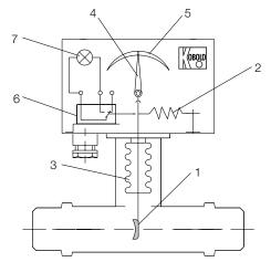
The motion is transferred positively from the baffle (1) to the measuring section.
