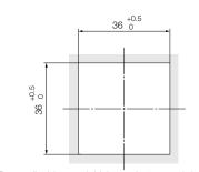
The applicable panel thickness is 1 up to 3,2 mm
